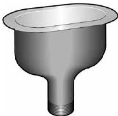
0975-0F Stainless Steel Made of type 316 stainless steel and has integral cross bars. 6"x 3" I.D. 1 1/2" I.P.S. male straight thread outlet.
