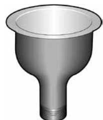
0950-0F Stainless Steel Made of type 304 stainless steel and has integral cross bars. 5" I.D. 1 1/2" I.P.S. male straight thread outlet.
