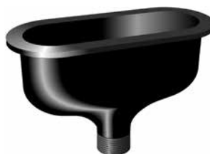
0492-BP Black Poly 0492-GP Grey Poly Complete with removable strainer. 9"x 3" inside dimension. 1 1/2" I.P.S. male straight thread outlet. (Overall height is 7")
