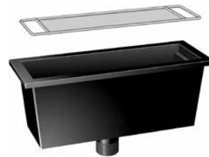
0493-BE Black Epoxy 0493-GE Grey Epoxy 0493-PE Putty Epoxy 0493-SE Slate Epoxy Complete with removable type 316 stainless steel wire screen. 13 3/8"x 4 1/8" x 5 1/4" I.D. 1 1/2" I.P.S. male straight thread outlet. (Overall height is 8")
