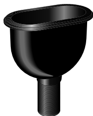
0491-BP Black Poly 0491-GP Grey Poly Complete with removable strainer. 6"x 3" inside dimension. 1 1/2" I.P.S. male straight thread outlet. (Overall height is 8 1/2")
