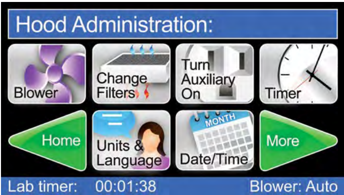
AirSafe NXT allows the operator to set language preferences and display unit of measure preferences
